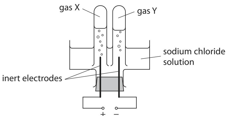
During the electrolysis two gases, X and Y, are formed. One of the gases produces a squeaky pop when tested with a lighted splint.
